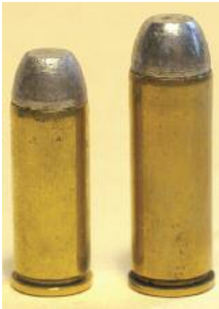
Comparative view of modern .44 Colt (left) and .45 Colt (right)
