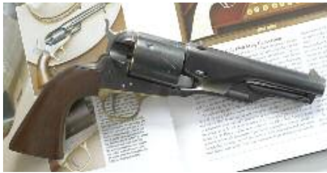
Centaure Marshal #12089 converted in 2010 by German gunsmith Klaus Mumme into a Long Cylinder Conversion chambered for .44 Colt. Note straight cylinder. Originals chambered for .44 Henry rimfire were probably made by gunsmiths in Mexico about the same time Colt manufactured their Thuer conversions during the late 1860s.
