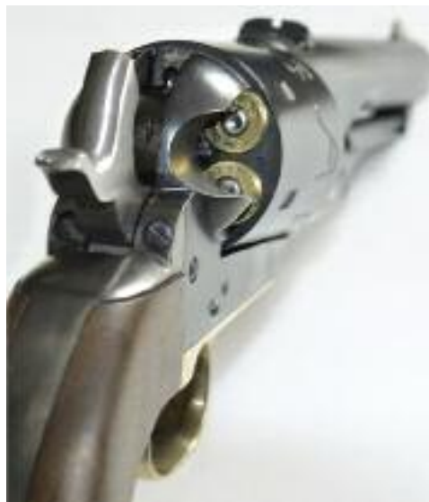
Like the originals, the Centaure Long Cylinder Conversion has no loading gate. That works fine as long as you are not cocking the pistol while aiming at the sun! Similar to the later Colt Open Top, a number of these Long Cylinder Conversions had their rear sight dove tailed on top of the barrel.
