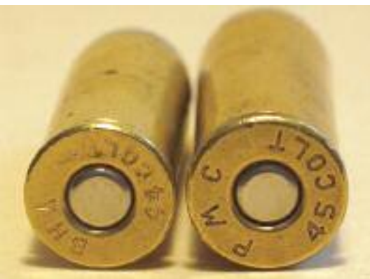
Smaller rim of .44 Colt (left) compared to .45 Colt (right)
